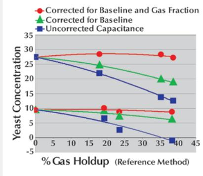
fermentation. The instrument also can measure the actual gas hold up in the fermentation, providing customers with an additional useful measurement parameter (e.g. onset of foaming). The multifrequency system is used to calculate the true fraction of biomass present regardless of gas distribution. Figure 3 shows an example of how the
