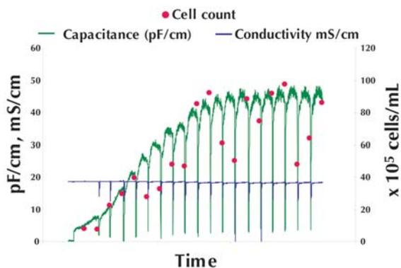
**Figure 10:** Monitoring an Escherichia coli fermentation by RF impedance, optical density, and plate counts in a pilot plant 2,000-L fermentor (units have been normalized).
