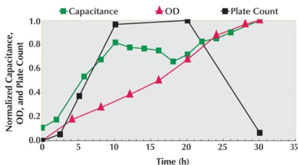
Yeast Monitor can reveal a unique yeast growth and flocculation profile. The capacitance trace not only provides valuable information on the cell concentrations after seeding and transfer to the next stage, but a change in the profile will also provide valuable feedback on any upstream changes in the quality of the media (brewers' wort) feed.
