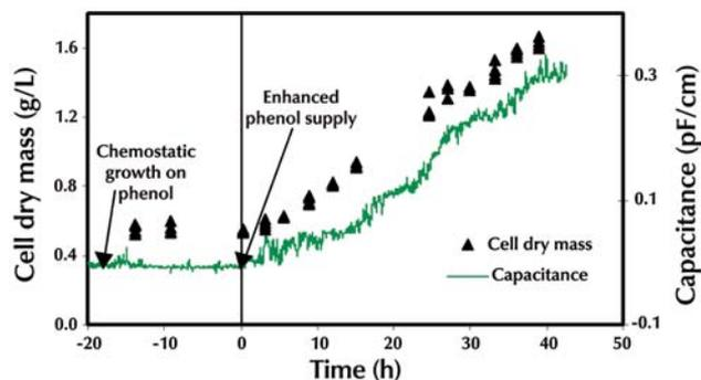
**Figure 11:** Monitoring a production yeast fermentation by RF impedance: capacitance has been converted to cells/mL.
