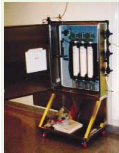
Photo 2: Prototype chlorine dioxide gas generator showing CD-generating cartridges
