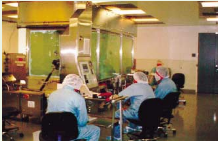
Photo 1: Aseptic fill isolator undergoing chlorine dioxide disinfection
