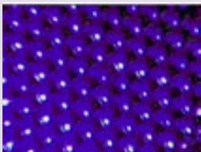
Photo 3: Monodisperse polymer hydrogel microparticles ( $400\ \mu\text{m} \pm 1\%$ )
